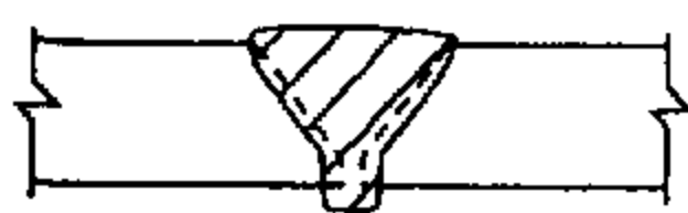
Single-V butt joint
