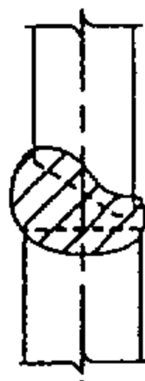
Angle-to-shell butt joint complete penetration
